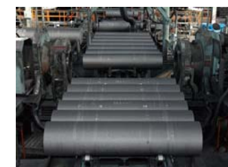
Machining line of Artificial Graphite Electrodes
